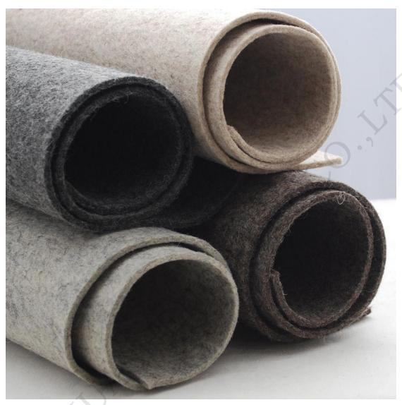
Needle punched felt refers to felt that is made by vertically needling fibers together to achieve a desired thickness and density. Needled felt is commonly made from wool, synthetic and other re-processed fibers. When viewing a cross-section of needled punched felt, the fibers lay vertically, as opposed to pressed felt, where the fibers lay horizontally.
